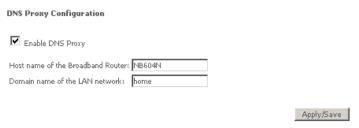
Enter your selected hostname and domain name for the DNS Proxy function and click Apply/Save to save the new DNS Proxy configuration settings.
