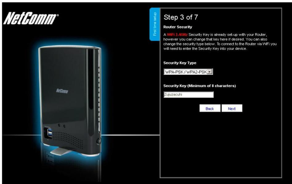
Figure 4 - Setup Wizard Step 3 – 2.4 GHz WiFi Security Settings
