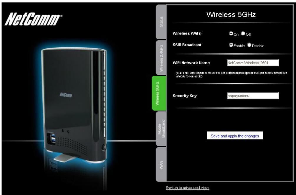
Figure 10: Basic - 5.0 GHz Wireless
