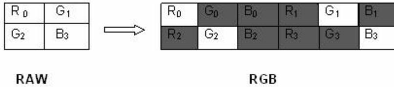
where the shaded values are to be calculated by the algorithm. Subscript denotes the tile on the Bayer Pattern to which the value of R, G, and B belongs. Note that the image size will become 3 times the Bayer Pattern. In order to view the RGB image we convert it to a Bit Map, or .BMP image, by adding a bitmap header.
