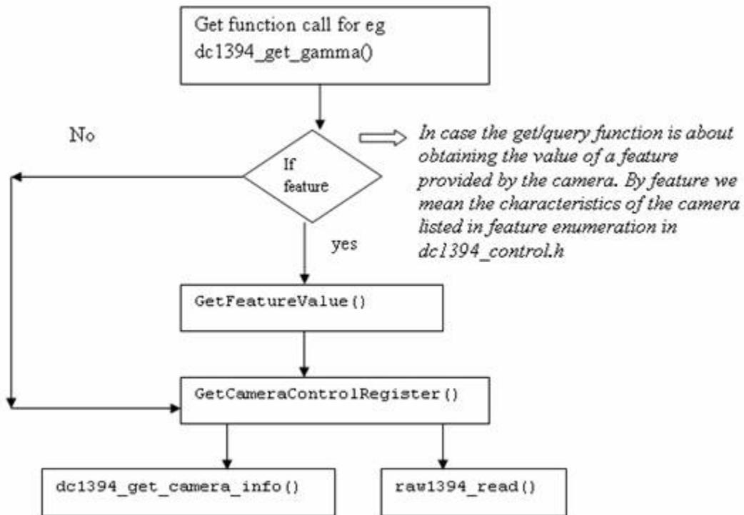
In case the `get` function you called is meant to retrieve the value of a camera feature (the value for the parameters listed in feature enumeration), that `get` function will call another `get` function (`GetFea-`
