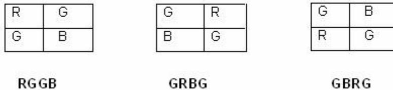
The image we obtained in the previous example was a Bayer Pattern image also known as a *RAW* image. This was stored in `camera.capture_buffer`. In order to view what we have captured we convert this RAW image to .PGM by adding a header (look at the explanation in the section called “Example: How to grab image from the IEEE1394 camera”).
