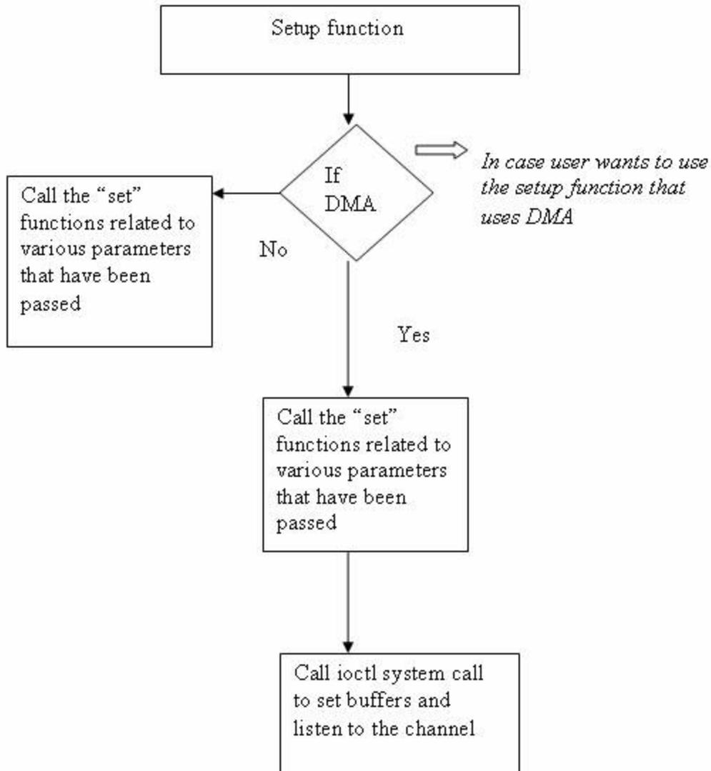
As shown in Figure 3, the Setup function in turn calls various set functions to set the parameter values to the camera registers. In the case of DMA setup, after the set functions have been called the ioctl system call is called to allocate memory for the DMA buffers and returns a pointer *capture\_buffer* in user space.
