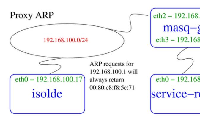
The device performing proxy ARP (masq-gw) responds for all ARP queries on behalf of IPs reachable on interfaces other than the interface on which the query arrives.
